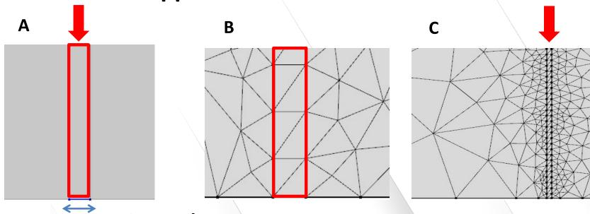
Fracture zone width: 3x10<sup>-4</sup> m where constant temperature is applied
